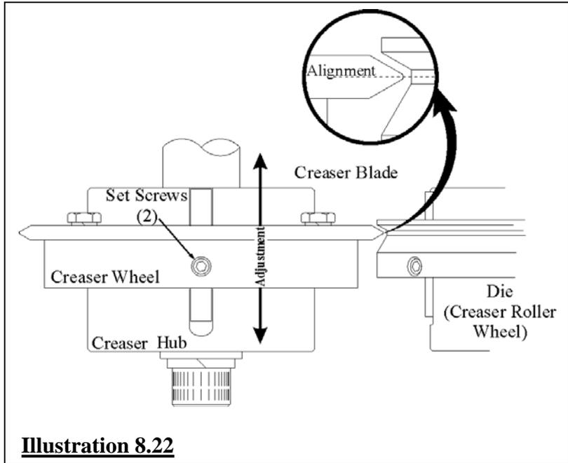
**(D). Setting the Gap: Blade Horizontal Adjustment**
