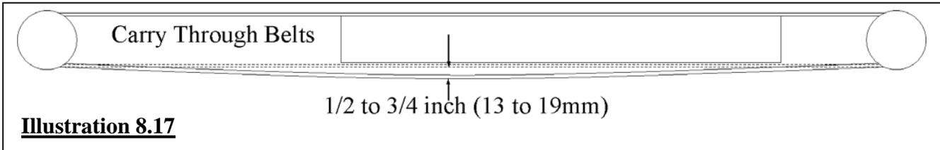
15. Once the tension is set, tighten the four top and bottom holding bolts on both infeed plates. **Section 8.5.2, page 30**
