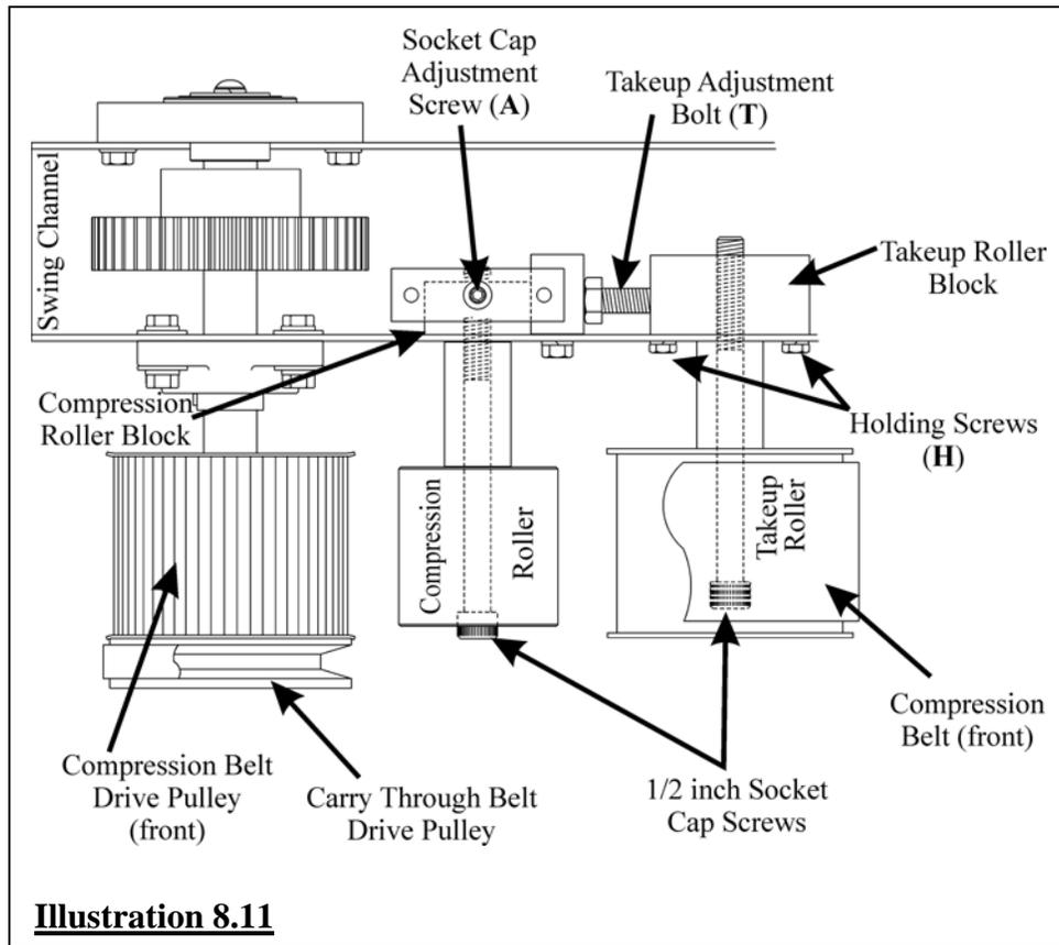
6. Push in on the belt between the takeup roller and the drive sprocket. If the tension in the belt is correct, the belt should deflect about  $\frac{1}{2}$  to  $\frac{3}{4}$  inch (13 – 19mm). (**Illustration 8.10**)
