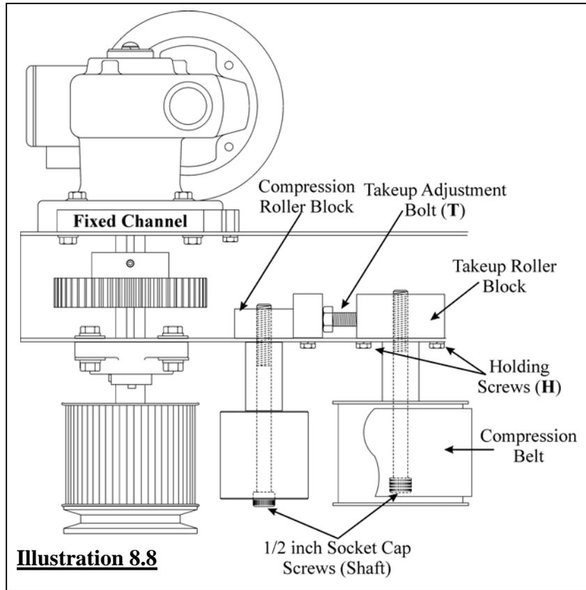
6. Secure the compression assembly in place by tightening the ½ inch socket cap screw (shaft). Double check the alignment of the compression belt after the screw is tightened. (**Illustration 8.8**)
