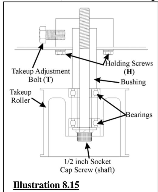
4. Loosen the ½ inch socket cap screws (takeup block only). (**Illustration 8.15**) This is done from the bottom of the rollers. Do not remove the screws.
