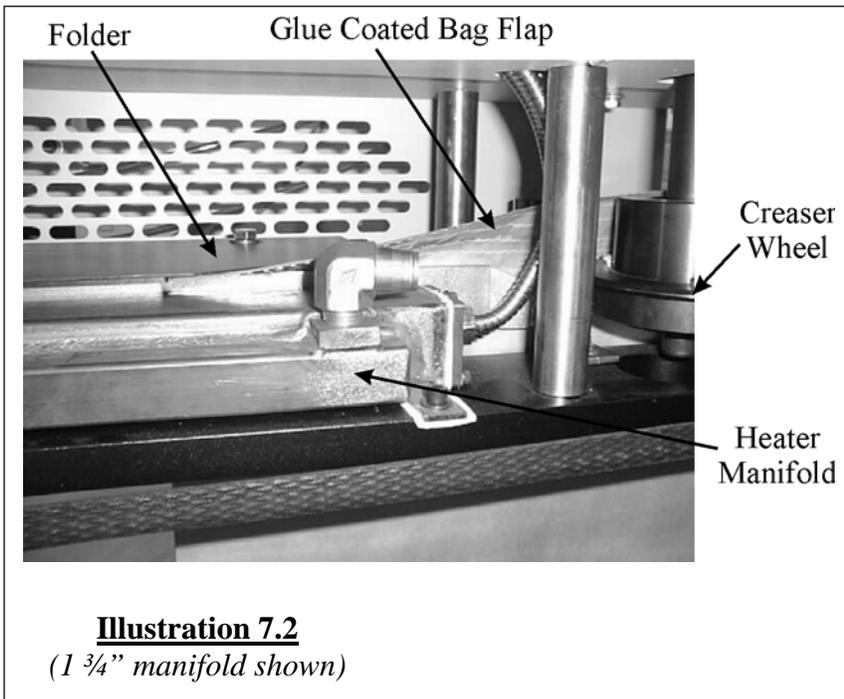
After the manifold, the folder continues bending the heated flap another 90° to complete the fold. The adhesive begins to make contact with the outer bag surface as the fold is completed and the bag enters the compression area of the machine. The wide compression belts guide the bag top between the compression belts. The belts press the flap firmly against the bag, to force the adhesive to penetrate the bag fibers. The completed fold and compression yield a sharp, clean fold with a strong bond.
